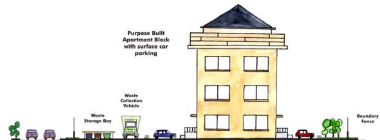
DESIGN 1: Apartment Block with open waste storage bay
